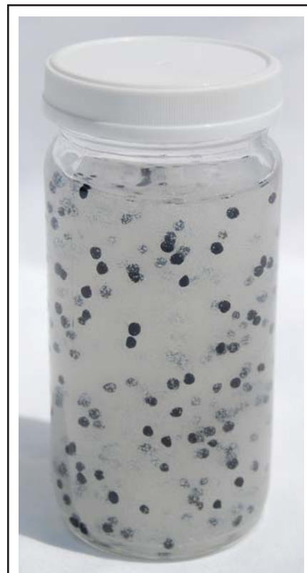
Halliburton is testing a new plastic-based ultralightweight proppant with a specific gravity of 1.08 g/cc in trial applications with temperatures to 200 degrees and up to 8,000 psi of closure stress. The proppant in this jar has been suspended in fluid for several days with no settling.
