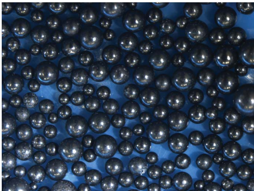
LiteProp™ 108, an ultralightweight thermal plastic nano-composite manufactured for BJ Services by Sun Drilling Products, has a nominal specific gravity of 1.054 g/cc and is engineered to withstand 225 degrees and 6,500 psi of closure stress.
